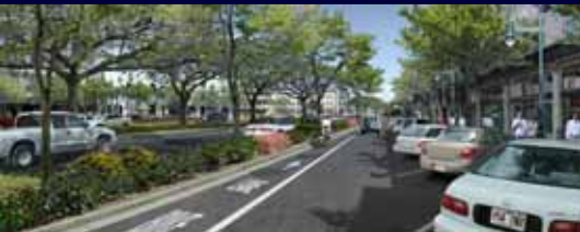
Alternative with two lanes each way for through traffic and service lane with diagonal parking
